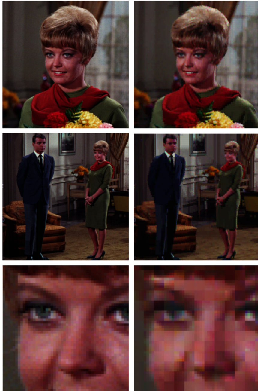
Fig. 4. “Girl” and “Couple” color test images, reconstructed images using the spread PFNN with 128 codevectors each plane, and their local enlarged images for the original and compressed images: original images (left), reconstructed images (right).
